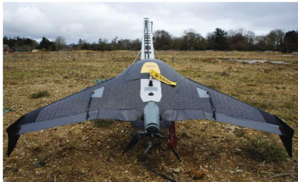
Ready to launch, the UX5 drone was developed as an early photogrammetry UAV.
