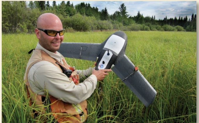
LW Survey Canada Chief Pilot Zak Bland recovers the X100 after a flight. The aircraft automatically descends and lands at a specified location.
