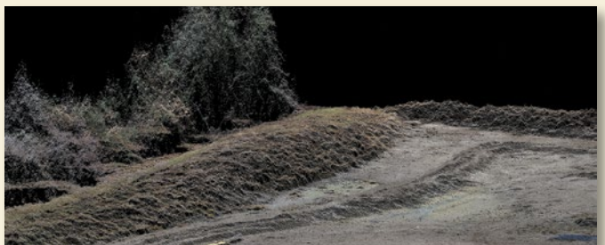
A colorized 3D point cloud from the Taiga site. The 3D model was developed using aerial imagery from the Trimble UX5.
