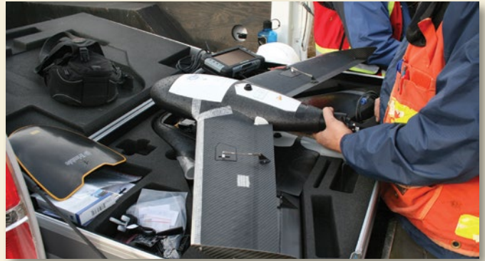
Robicheau compares the X100 and UX5 airframes. The UX5's larger wing area allows for better flight performance and shorter landings.
